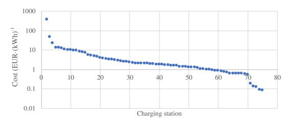
Fig. 1. Average cost of transmission and distribution per kWh charged in Latvian national fast charging network
